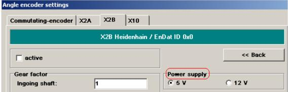
Figure 7: Metronix ServoCommander®: Angle encoder settings [X2B]
